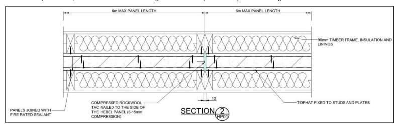
Figure 2 - Hebel party wall vertical joint with compressed rockwool
