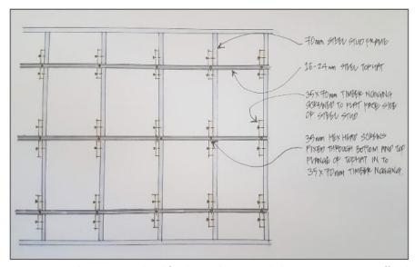
**Figure 4** –Proposed construction detail for the overhanging Hebel Intertenancy system affixed to a steel frame using timber noggins and top hats
